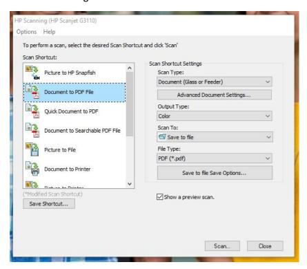
Press the "Scan ..." button again. The HP Scanning window opens. The window on the left provides a status message, "Preparing to scan..." There is a significant pause before the scanning starts. The scanner lamp turns on which is visible around the edges of the scanner lid. The motors that move the scanning bar start up.
