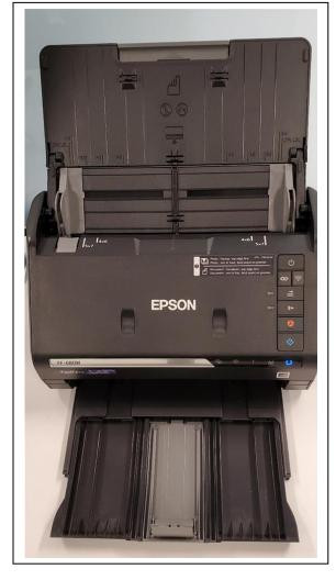
To scan, sort your pictures into sets with the same width, place them in the scanner between the adjustment guides with the picture side facing you and top of the picture pointing down (upside down). Then adjust the guides to snugly fit the photos.
