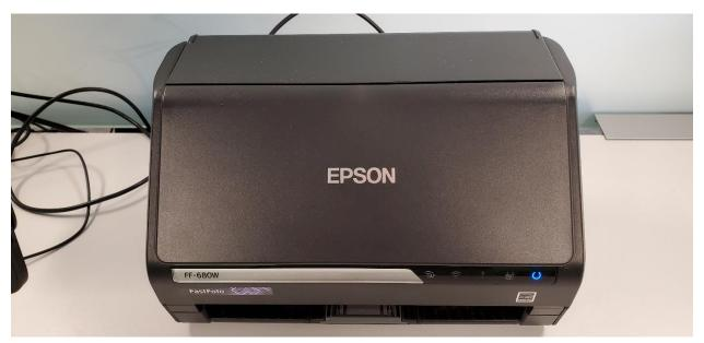
This is the Epson FF-680W FastFoto Scanner. In this picture the scanner doors are closed to protect it when moved or from dust. The FastFoto scanner scans photographs and is equipped with an Automatic Document Feeder (ADF) which enables it to quickly scan up to 30 photographs in one operation. The scanner assembly is in a fixed location in the scan path. As the ADF moves the pictures through the path, the scan is captured. In addition, it has software that can optionally:
